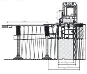
■ DRAINAGE PROFILE Width options: 120 and 170 mm, with galvanized or stainless steel grate
